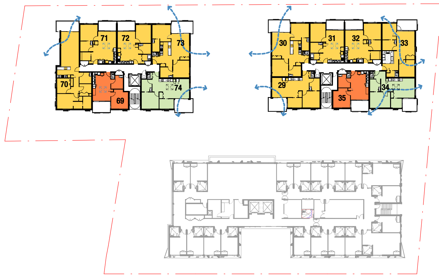
6 LEVEL 05 - SOLAR ACCESS & CROSS VENTILATION 1 : 500
