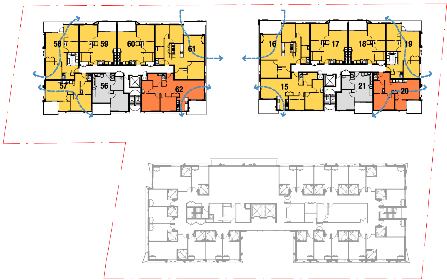
4 LEVEL 03 - SOLAR ACCESS & CROSS VENTILATION 1 : 500
