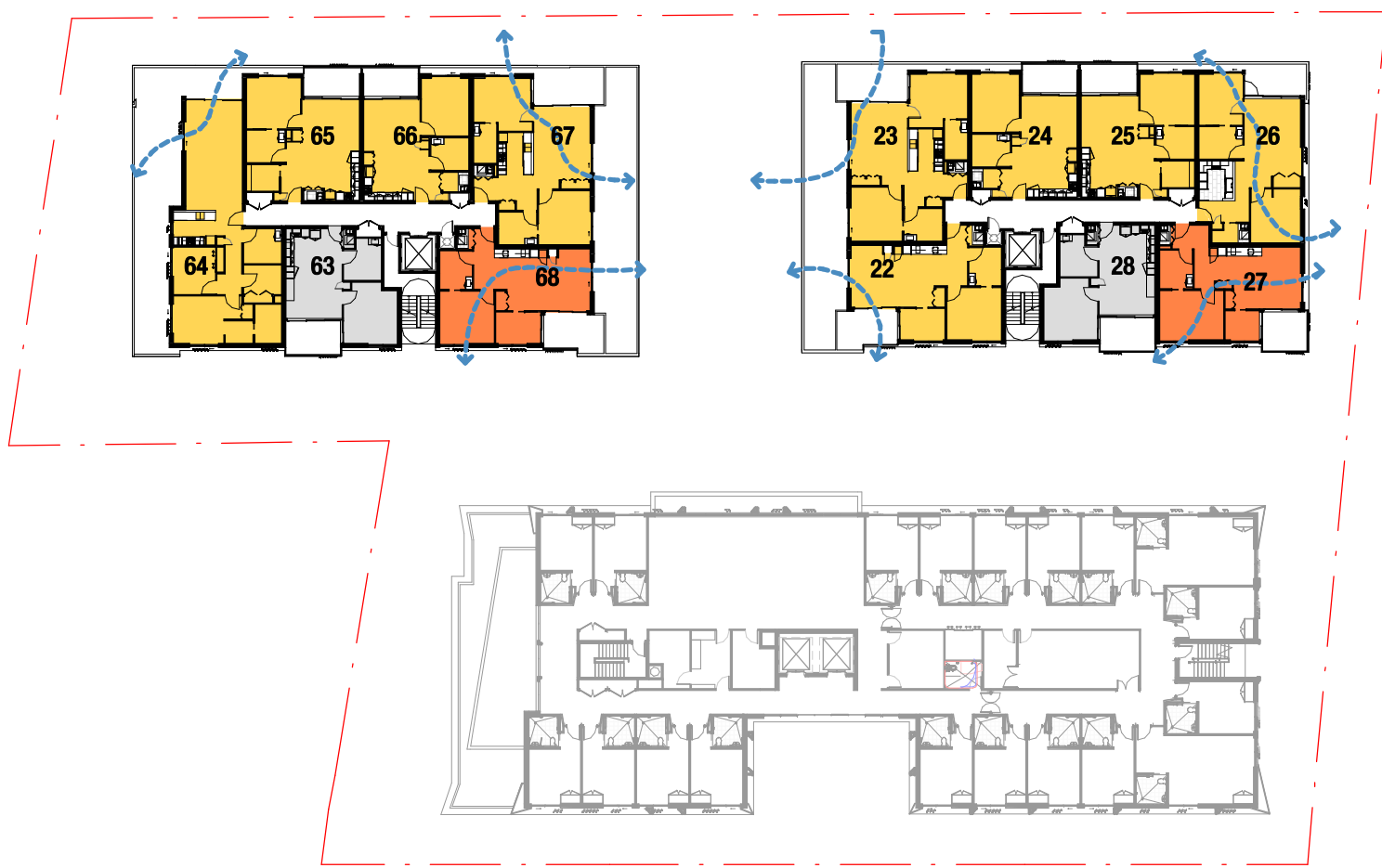
5 LEVEL 04 - SOLAR ACCESS & CROSS VENTILATION 1 : 500
