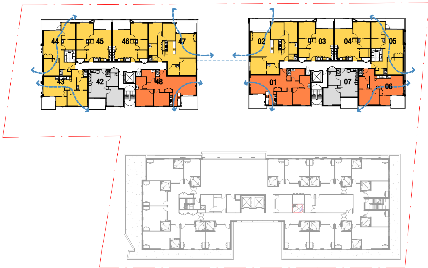
2 LEVEL 01 - SOLAR ACCESS & CROSS VENTILATION 1 : 500
