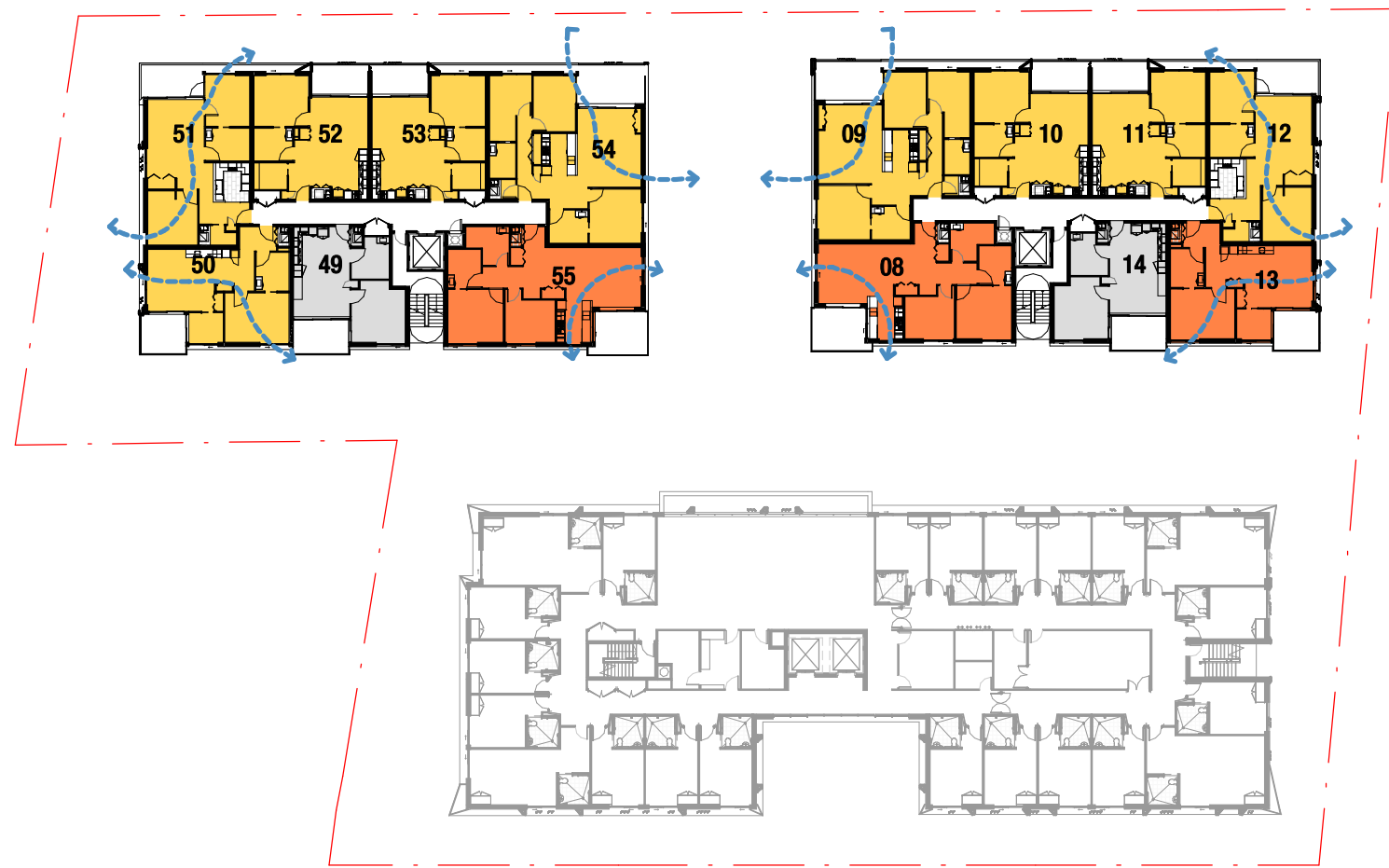
3 LEVEL 02 - SOLAR ACCESS & CROSS VENTILATION 1 : 500
